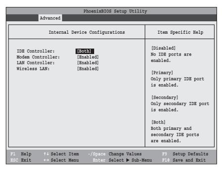
Figure 7. Internal Device Configuration Submenu
